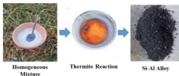
Figure 1: Aluminothermic Silicon Extraction Process.
