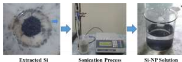
Figure 2: Mechano-chemical approach to synthesize Si-NPs.
