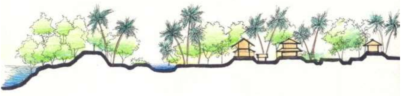
Figure 11- Section of a safer settlement showing Mangrove Forest, embankment and plantation. (Source: Islam, S. M. et al 2019)
