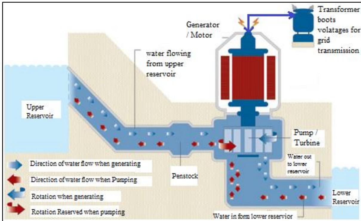
Fig. 5. Open-loop pumped storage hydropower plant arrangement [7]
