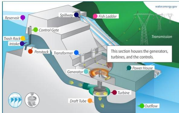
Fig. 2. The electricity generation process of PSH [7]
