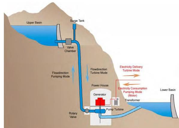
Fig. 4. Closed-loop pumped storage plant arrangement [3]
