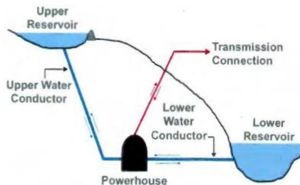
Fig. 1. Typical PSH Configuration [5]
